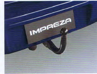
73. Trailer hitch Towing capacity maximum 1,600 kg.
