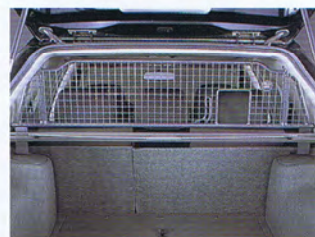
75. Dog guard (G/M) Separates cargo room from passenger area, applicable for ISO FIX child seat.
