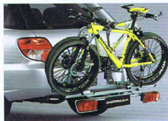
72. Rear bicycle holder (Installed on tow ball) Transports 2 bikes on tow ball.
