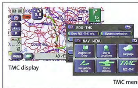
60 TMC unit (DVD Navigation) H001EAG102 W Provides traffic information and alternative routes avoiding traffic jams.
